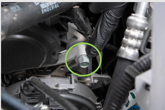
STEP 15 - Locate and remove the upper bolt of the iBSG
