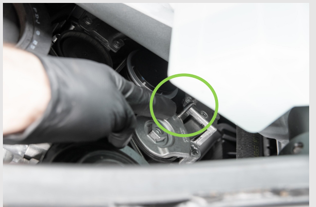
STEP 8 - Release the blocking tool in the tensioner to tension again the belt
