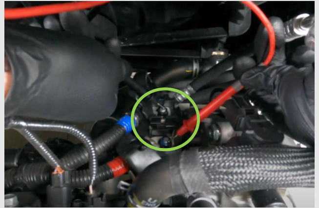
STEP 6 - Check with the multimeter the absence of current in the iBSG
