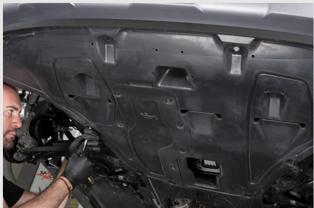
STEP 11 - Remove the lower engine cover
