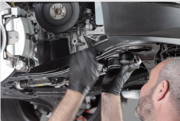
STEP 1 - Position the iBSG with the regulator part down
