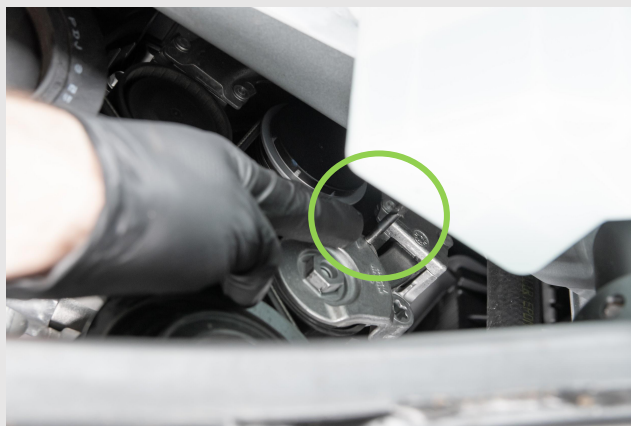
STEP 14 - With the belt tensioner loose, remove the belt
