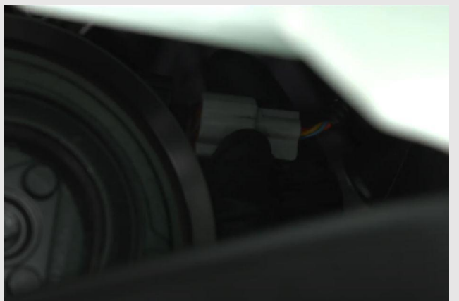
STEP 6 - Do not forget to plug again the electrical connections for the compressor
