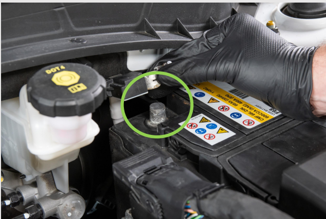
Step 1 - Disconnect (-) terminal from the 12V battery
