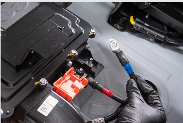
STEP 3 - Disconnect -48V terminal in 48V pack
