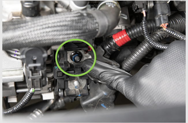
STEP 16 - Plug again +48V terminal in the iBSG
