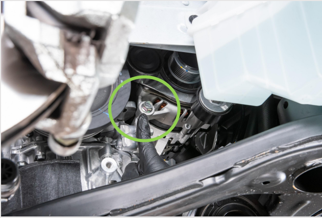
STEP 17 - Remove the lower bolt from the iBSG
