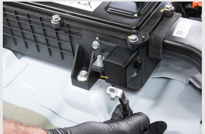
STEP 2 - Disconnect +12V terminal in 48V pack
