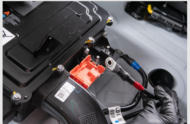
STEP 4 - Disconnect +48V terminal in 48V pack
