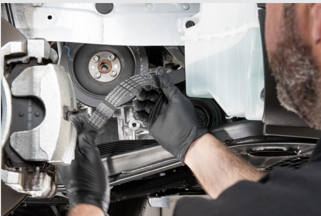
STEP 7 - Place the belt in the correct position defined by the car maker (it's recommended to install a new one)
