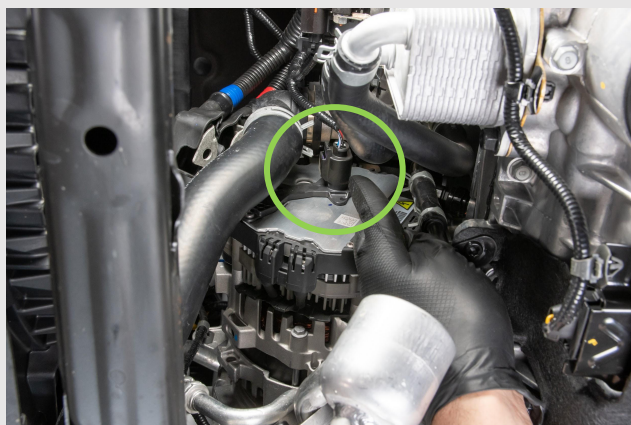
STEP 16 - Disconnect the ECU connector from the iBSG
