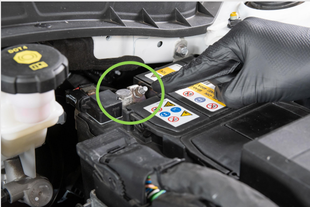
STEP 17 - Plug again (-) terminal from the 12V battery
