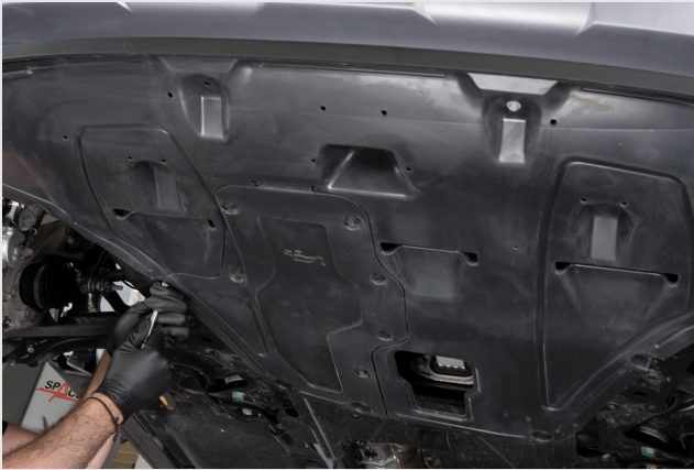
STEP 9 - Install again the lower engine cover
