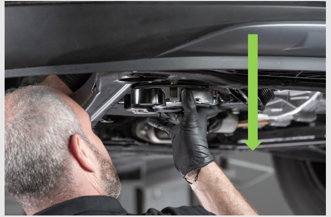
STEP 18 - Rotate the iBSG & take it out with the regulator part down
