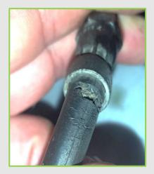
1. Age and wear: Over time, hydraulic brake hoses can experience degradation and wear due to exposure to heat, chemicals, and mechanical stress. This can lead to the development of cracks in the hose material.
