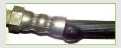
The presence of bubbles in the reinforcement of hydraulic brake hoses can occur due to a phenomenon known as "cavitation."
