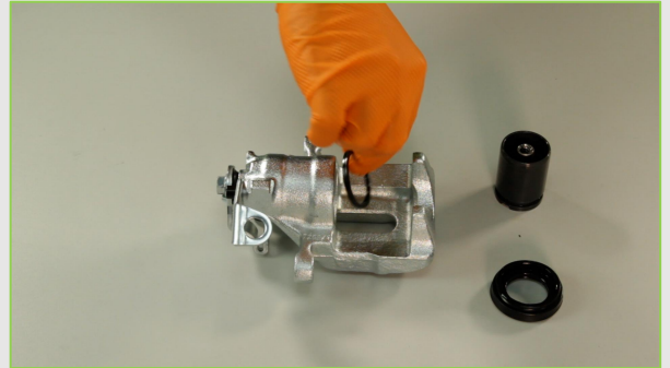
STEP 6 - Remove the outside piston seal inside the caliper
