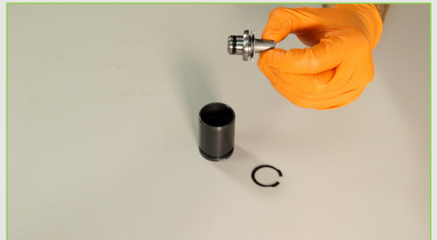
STEP 8 - Dismount the piston actuator screw
