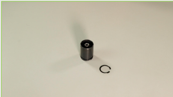
STEP 7 - Disassemble the seeger ring from the brake piston
