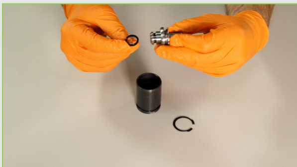
STEP 9 - Unclamp the seal from the piston actuator screw
