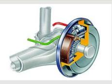
**Brake hose** is a **flexible** hose part in the braking system, that carries the **braking pressure** from the brake master cylinder to the brake wheel cylinder.
