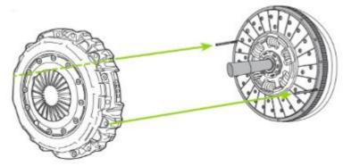
Please note; Valeo Service do not recommend the use of impact drivers to install clutch or flywheel bolts as torque tolerances can not be accurately respected.
