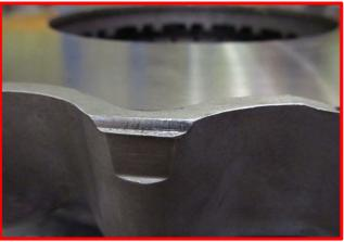
Valeo Service recommend using guidance installation pins when fixing CV clutch covers on their respective flywheels. This ensures that the clutch cover is in its accurate position. If the clutch cover is damaged, it should not be refitted.
