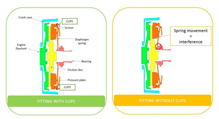
REMOVE THE SHIPPING CLIPS AFTER ALL COVER BOLTS HAVE BEEN FITTED.
