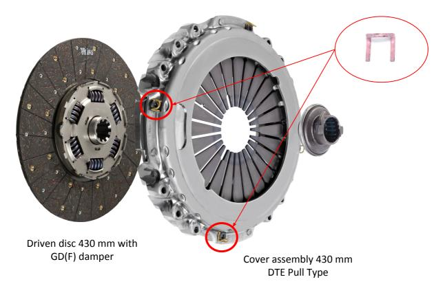
If the clips are removed prior to bolting the cover assembly to the flywheel, it can cause the pressure plate fingers to drop and potentially foul the friction plate.
