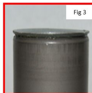
The piston retaining ring has deformation or rippling. This shows that the cylinder has been overstroked.
