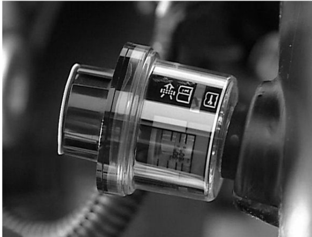
Figure 24 Air Cleaner Restriction Gauge (Courtesy of Jim Halderman)
