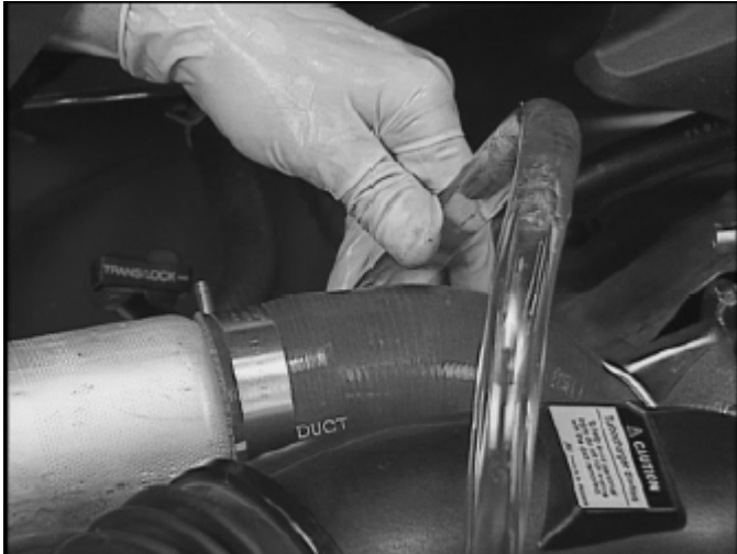
Figure 78 Clear plastic hose in the SUCTION side (Courtesy of GM)
