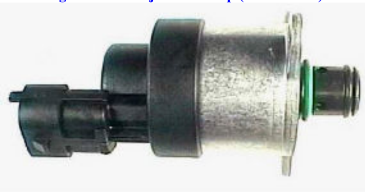
Figure 5 LB7 Fuel Rail Pressure Regulator (FRPR) valve (Courtesy of Jim Halderman)
