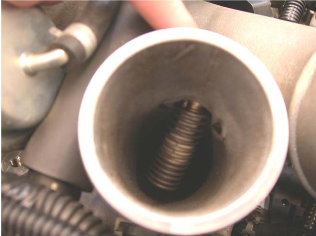
Figure 23 LB7 Intake Air Heater (Courtesy of Jim Halderman)
