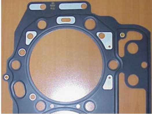
Figure 18 2006 Riveted Head Gasket Design
